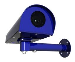
The **NC5** is designed and approved for use in hazardous (explosive) gas atmospheres that may be encountered in coal mines. It carries both ATEX and IECEx accreditation and is certified intrinsically safe to Group I (Ex ia 1 Ma) and also tested to **IP65**.
